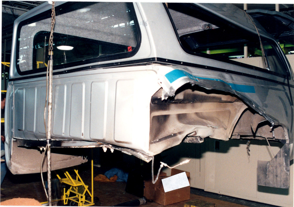
6. Left side of the cargo bed showing the damaged side panel resulting from the CNG tank failure and post event alteration
